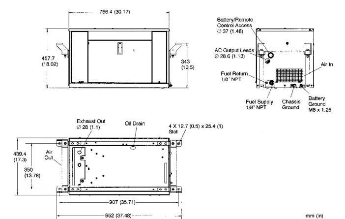
**Note:** This outline drawing is provided for general reference only and is not intended for design or installation. For more information see Operation and Installation manuals or obtain 500-4709 drawing and wiring diagram from your distributor/dealer.
